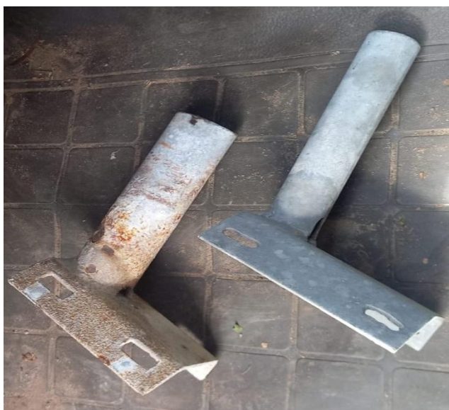
Wooden pole brackets(19mm strapping)
