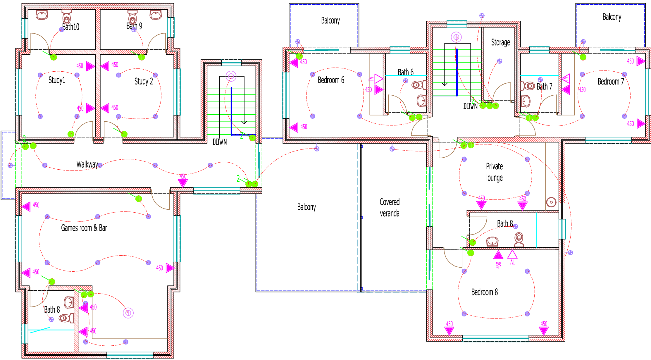
ELECTRICAL LAY-OUT - FIRST STOREY SCALE 1:100
