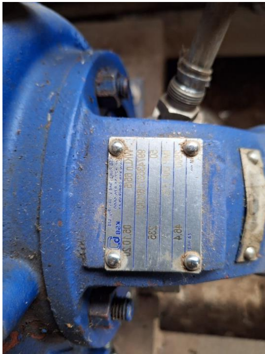
KSB WKLn G5/5 Impeller 235mm RPM 2 900
